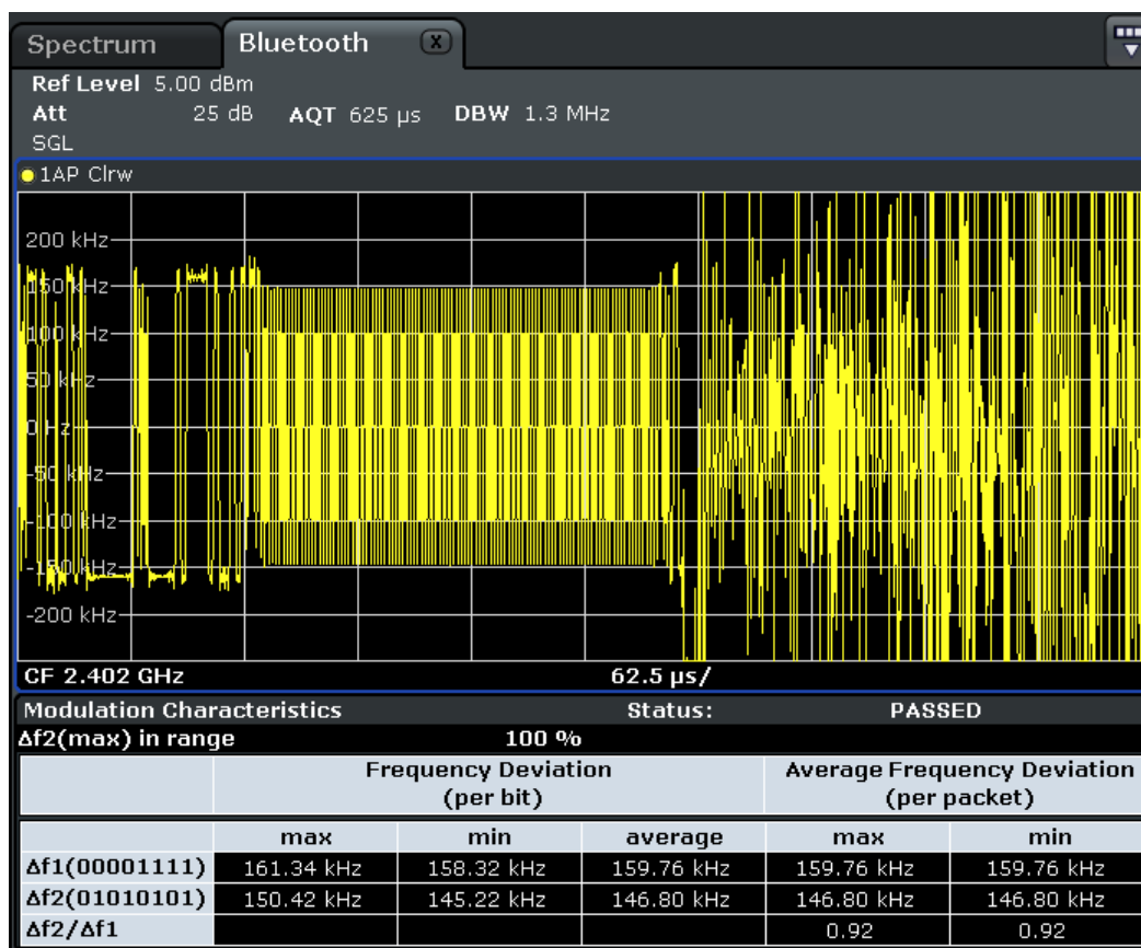
Fig. 4-4: Modulation Characteristics measurement
